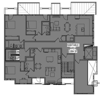
3 Floor Area Ratio Diagram, Level 3
