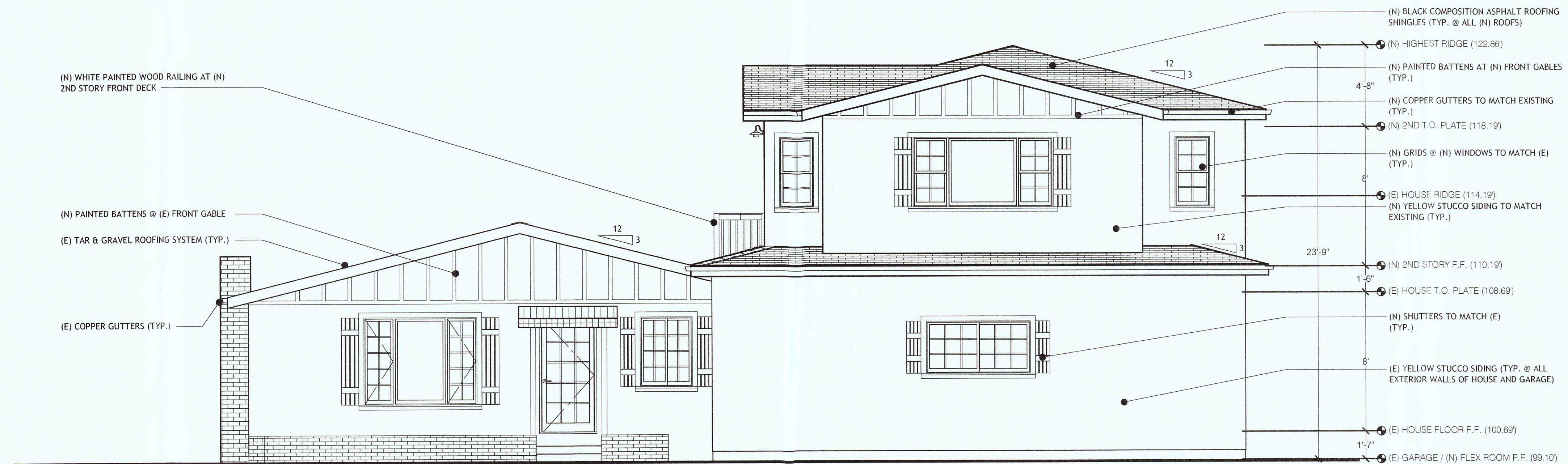
2 A4.1 PROPOSED FRONT (SOUTHEAST) ELEVATION SCALE: 1/4" = 1'-0"
