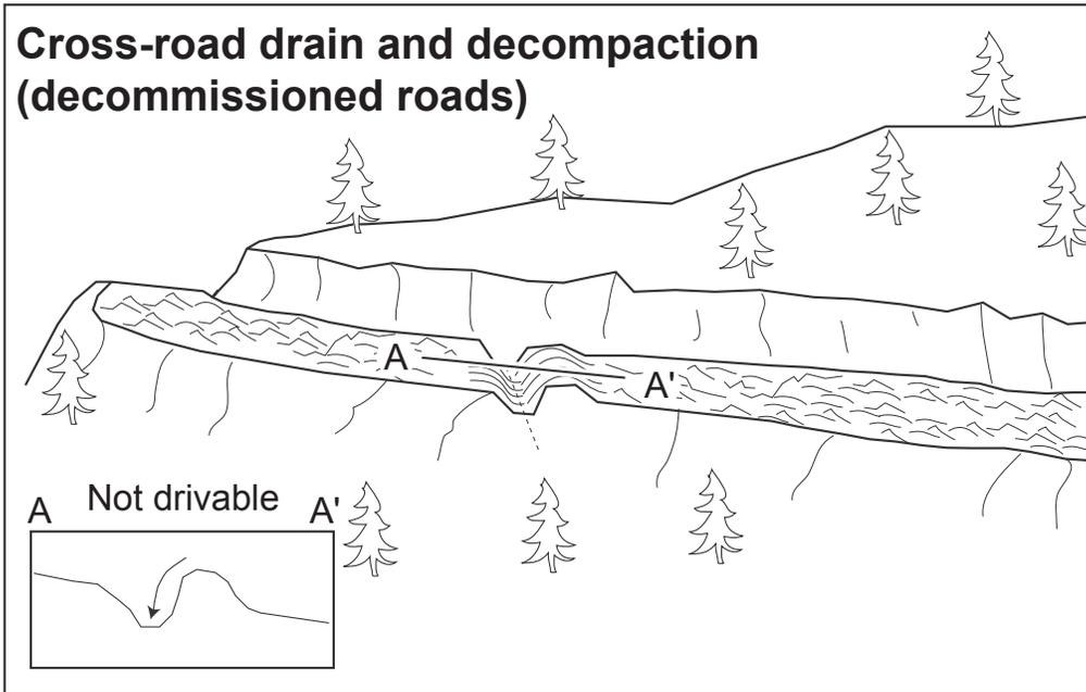
*Cross road drain* construction will ensure gullies, springs, road runoff and other concentrated flow will no longer collect over long lengths of road causing gully erosion and sediment delivery to streams. Cross road drains will be constructed at approximately 75 ft spacing intervals and these cross road drains will direct road surface runoff off the road onto stable hillslope locations.
