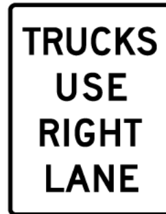
Figure 9: Trucks Use Right Lane Signage (R4-5)
